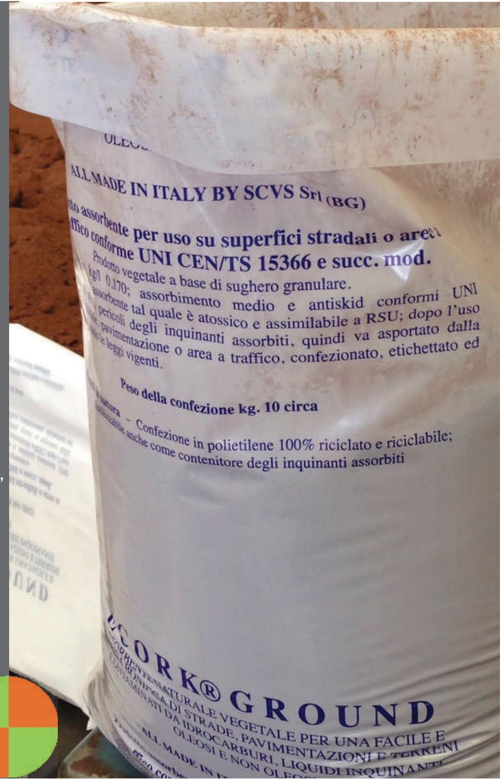
*Loose granulated cork of a diameter up to mm 1.5 c/a and unit weight of 0.18-0.30 kg/l c/, made from natural cork; it is suitable for absorbing hydrocarbons and oily pollutants spilled on floors, streets, and roadways.*
